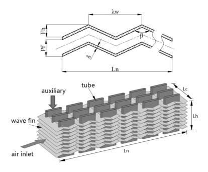
Fig. 1. Wavy fin: top–geometric parameter, bottom–structure of the fin and tube radiator  $% \left[ {{\left[ {{{\rm{T}}_{\rm{T}}} \right]}_{\rm{T}}}} \right]$
